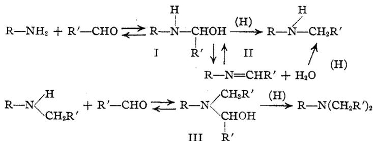
It cannot be said definitely that the amino alcohol (I) is reduced directly as suggested by Wallach<sup>3</sup> or that it is dehydrated to the Schiff base (II) before reduction. In either case the product would be the same, and it is quite possible the reaction follows both courses. Schiff bases have been reduced catalytically to secondary amines.<sup>5</sup>
